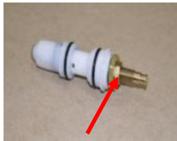
4. Adjust Cartridge by Loosening Hex Nut.
