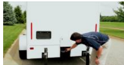
Accessible 4" Clean Out Port.
