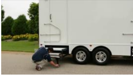
5. Pull Down Right Front Stair Jack.
