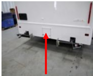
Accessible 4" Clean Out Port.
