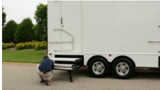
6. Pull Down Left Front Stair Jack.
