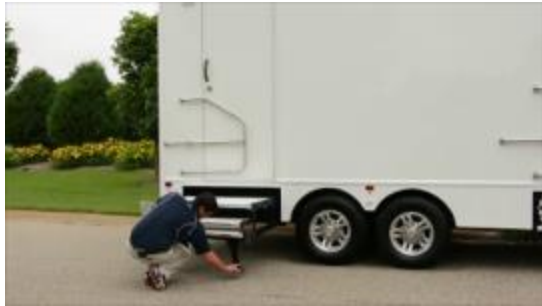
5. Pull Down Right Front Stair Jack.
