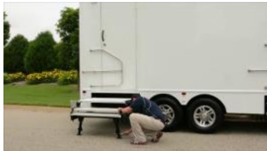
8. Add Tension with Service Area Bar.
