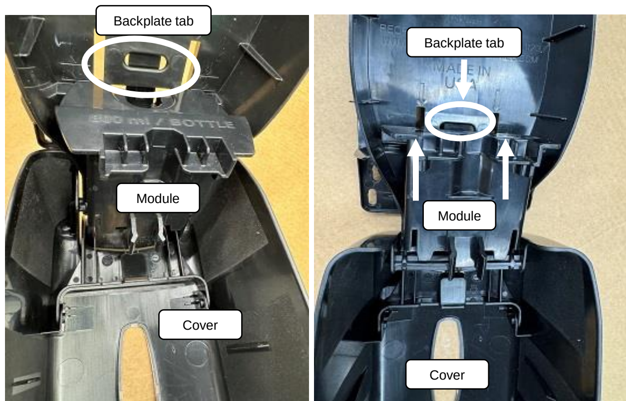
Remove module from backplate
