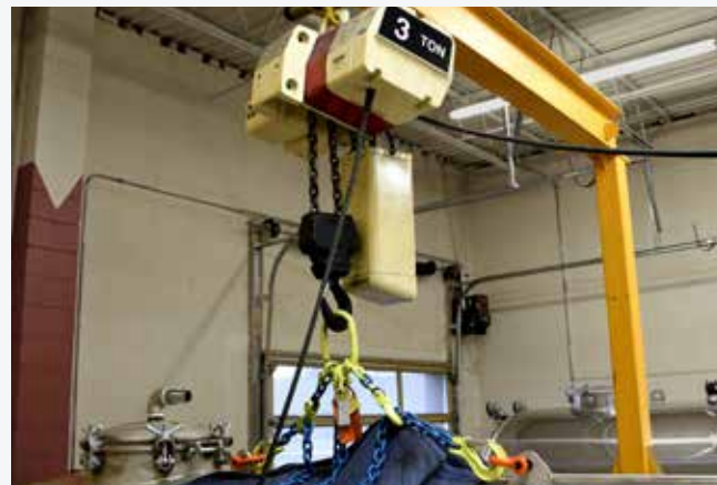
Figure 2.2 Hoisting Slide-in Unit for Installation in truck bed
